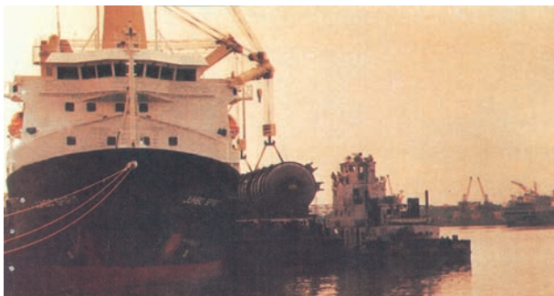
Fig. 7.8: Handling of oversize cargo at Tuticorin port
